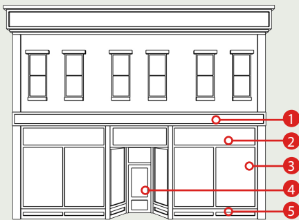
Figure 6.23: Typical Storefront Features
