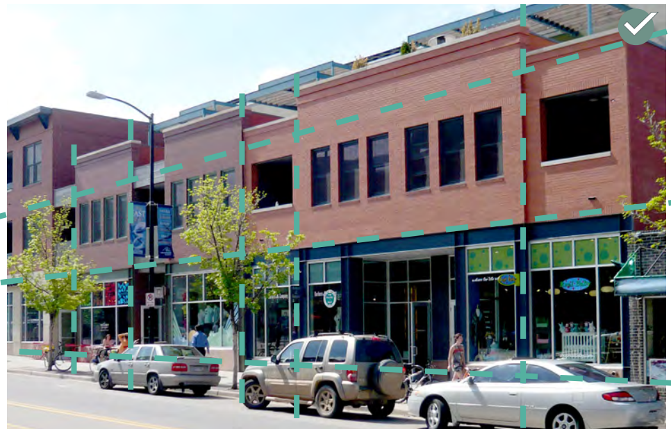
Design the first floor height to be taller than any upper floors and to appear similar in dimension to those seen traditionally.
