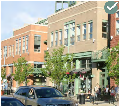
The massing of a parking structure should appear similar in scale to other active use buildings in the area. (This structure has an interior parking deck behind the “wrap” of articulated storefronts.)
