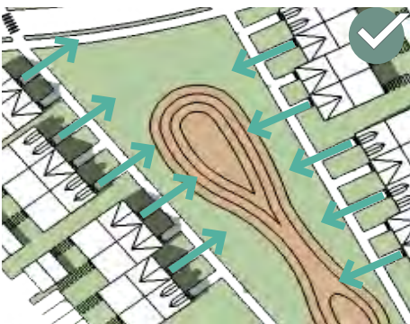
Figure 6.2: In multi-family development, place buildings to maximize common spaces shared between units.
