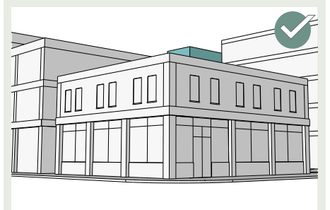
Locate rooftop elements to be sufficiently set back from the roof line so as not to disturb the cornice line of the building.
