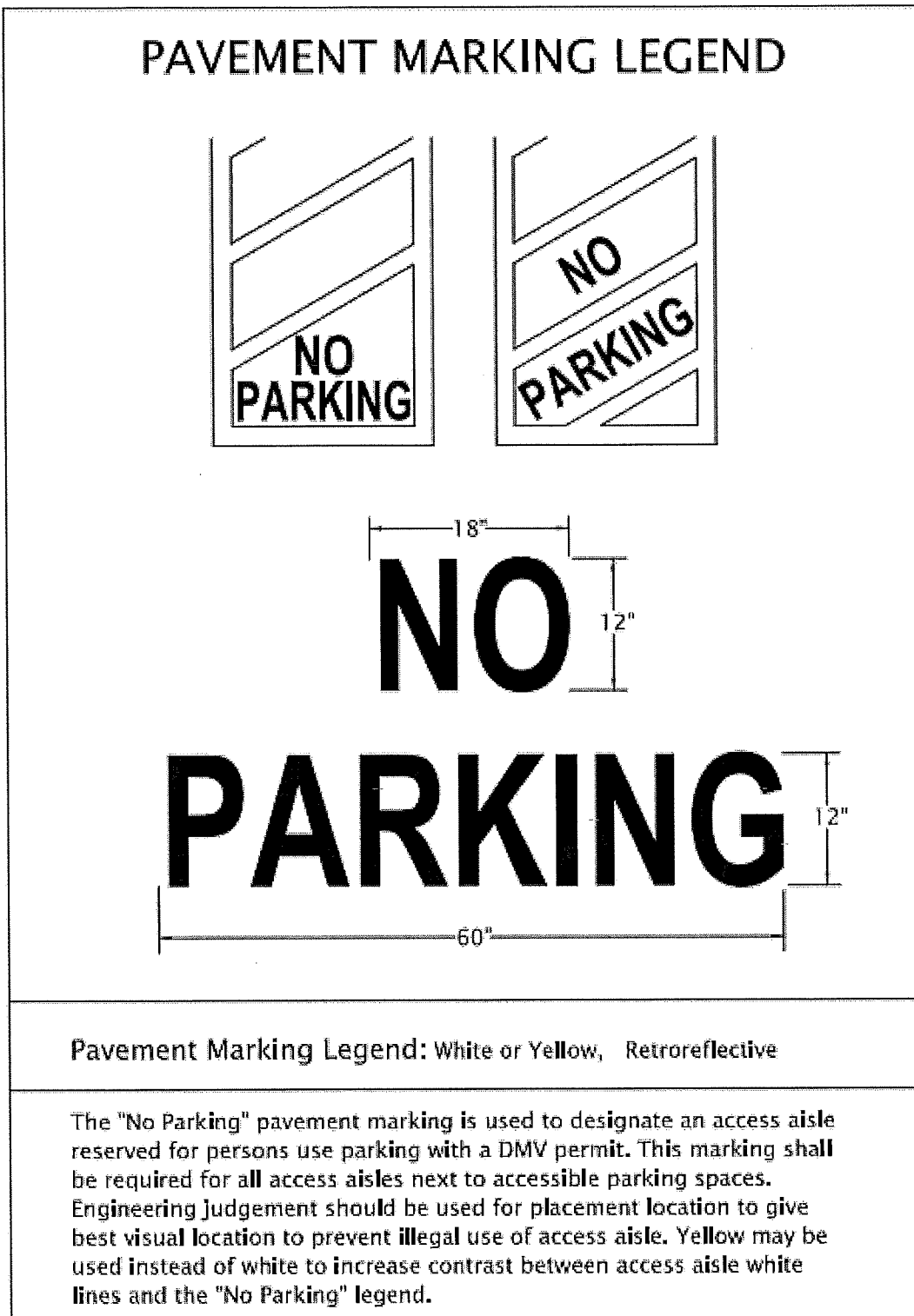
Figure 7: Pavement Marking Legend details for NO PARKING
