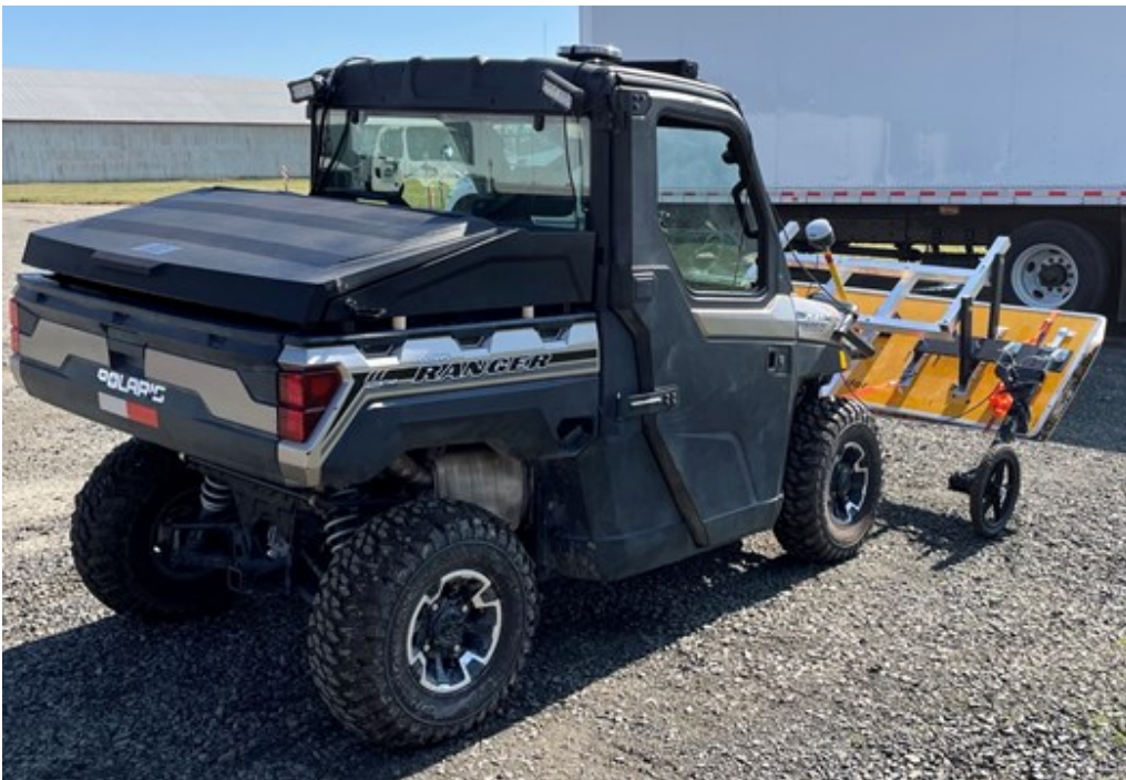
Multichannel antenna array collection vehicle, and sample data from historical trolley rail ties in Eugene OR
