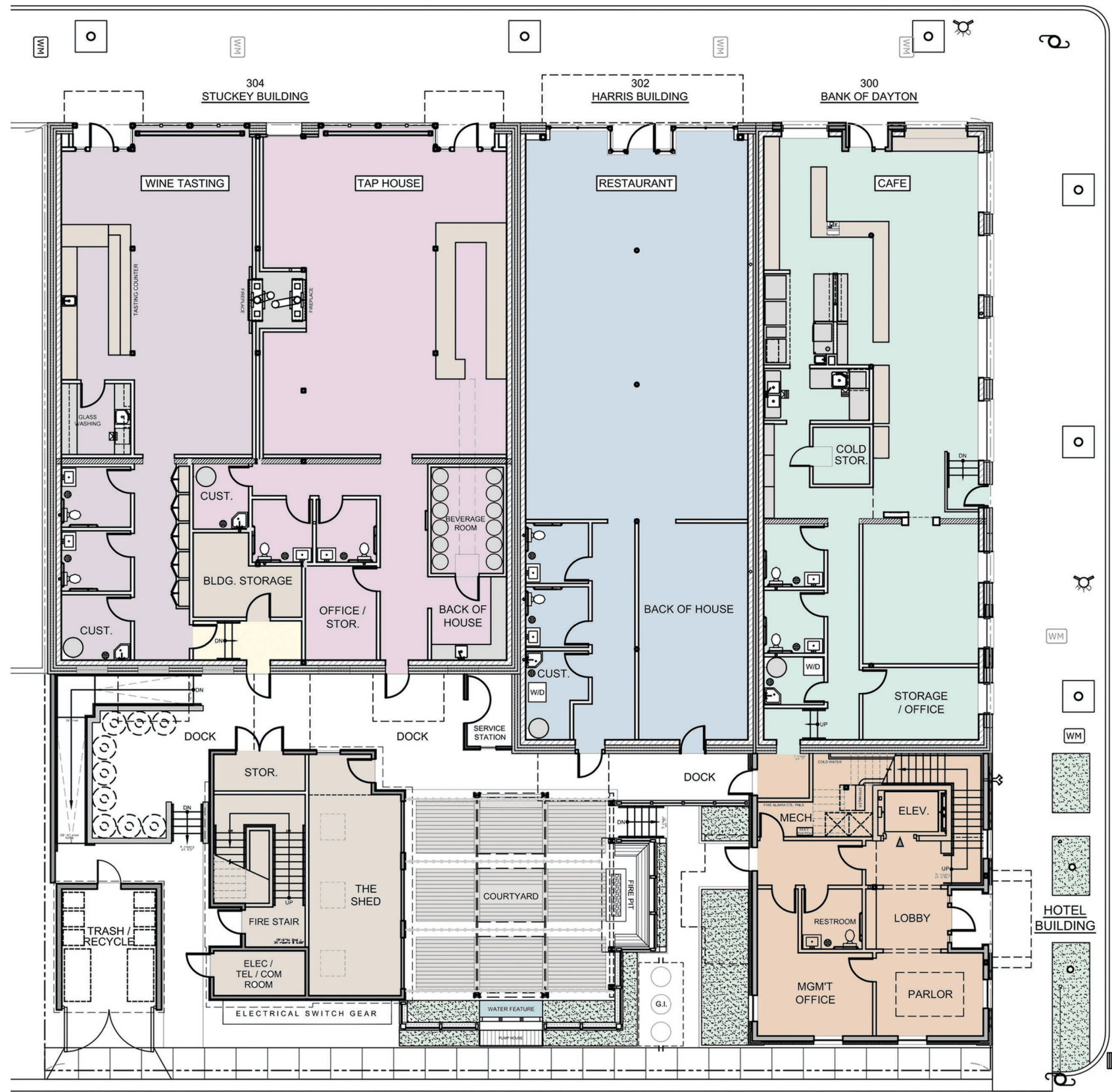
1 FIRST FLOOR PLAN SCALE: 1/8" = 1'-0" - half scale when printed at 11x17 -
