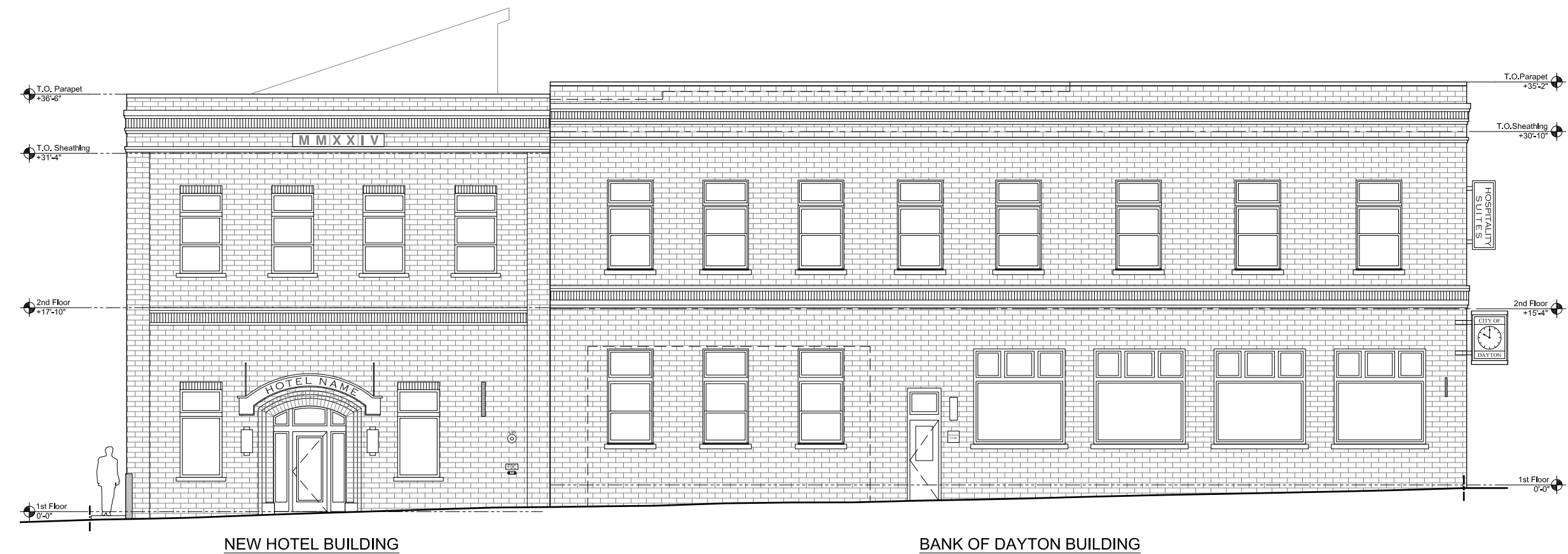
2 EAST ELEVATION [from 3rd Street] SCALE: 3/16" = 1'-0" - half scale when printed at 11x17 -
