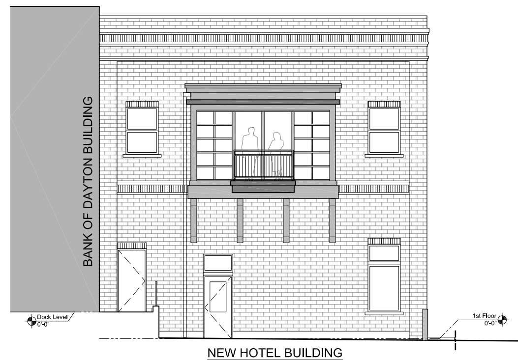
3 WEST ELEVATION [from Courtyard] SCALE: 3/16" = 1'-0" - half scale when printed at 11x17 -
