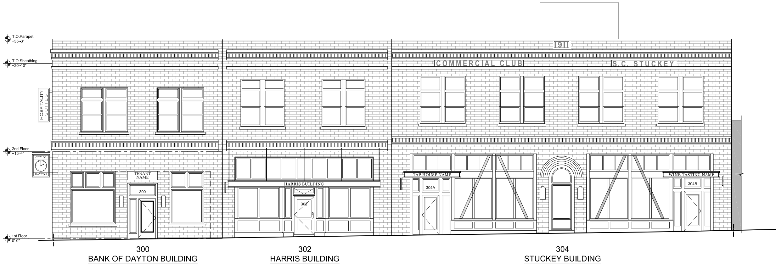
1 NORTH ELEVATION [from Ferry Street] SCALE: 3/16" = 1'-0" - half scale when printed at 11x17 -
